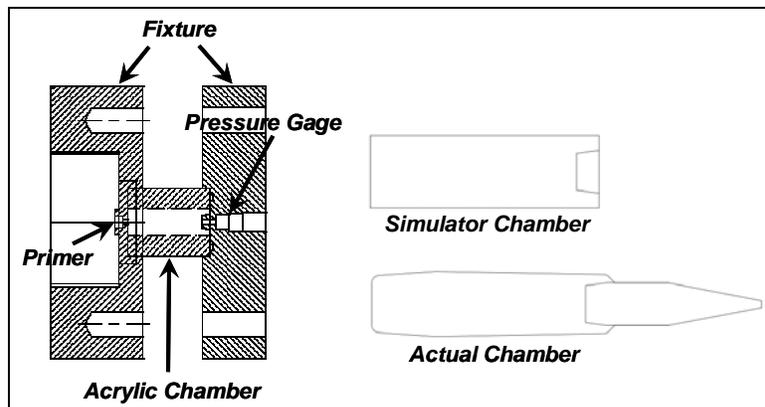
Figure 3. Schematic drawing of the 5.56-mm ballistic simulator.
