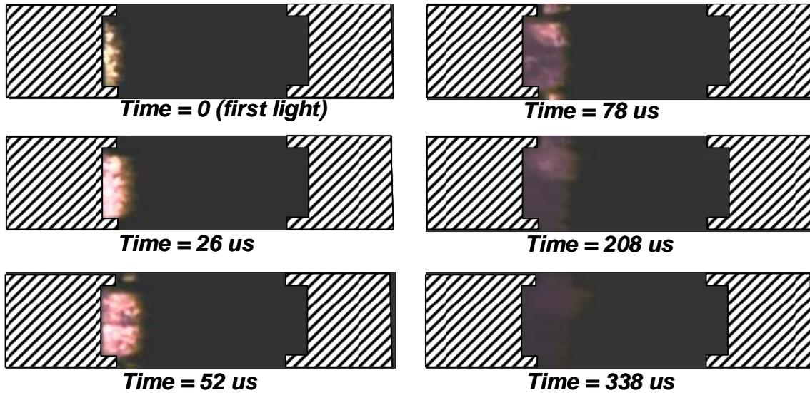
Figure 34. Flamespreading in live propellant bed (test 046).
