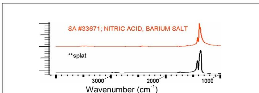
Figure 21. Reference spectrum of barium nitrate (top) compared to a spectrum representative (\*\*splat) of many residual particles from open-air firings. The y-axis is in units of relative intensity, and the main absorbance bands are at  $1420\text{ cm}^{-1}$  and  $1390\text{ cm}^{-1}$ .
