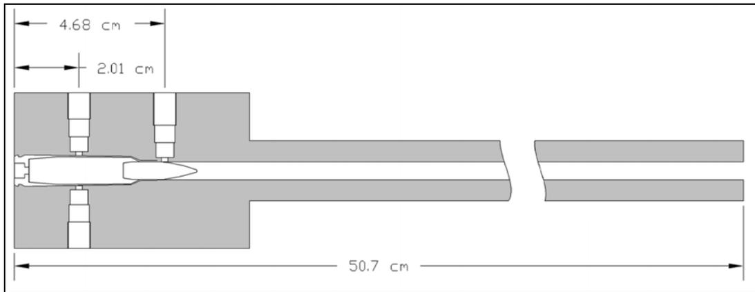
Figure 6. Schematic of gun firing fixture.
