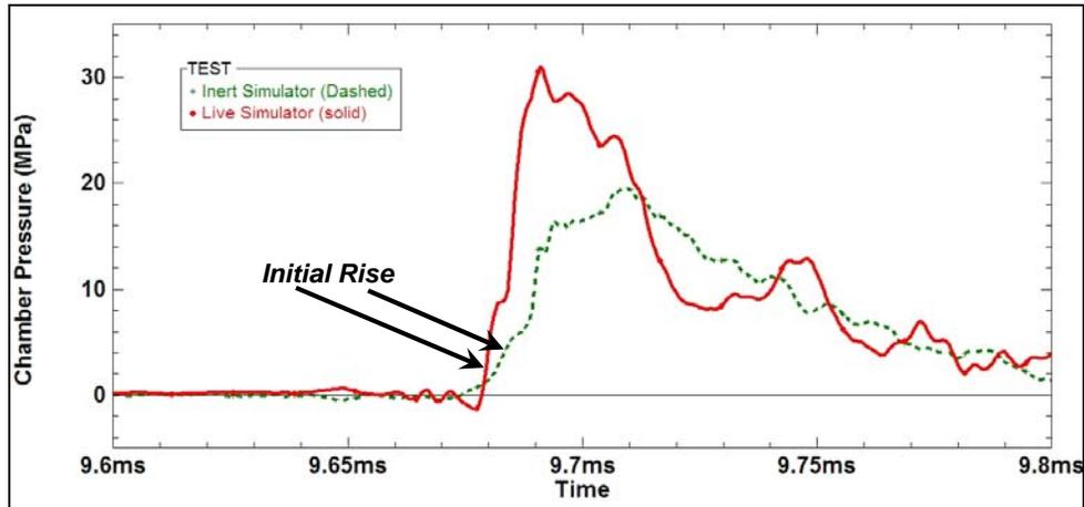
Figure 33. Live and inert simulator pressure-time traces.
