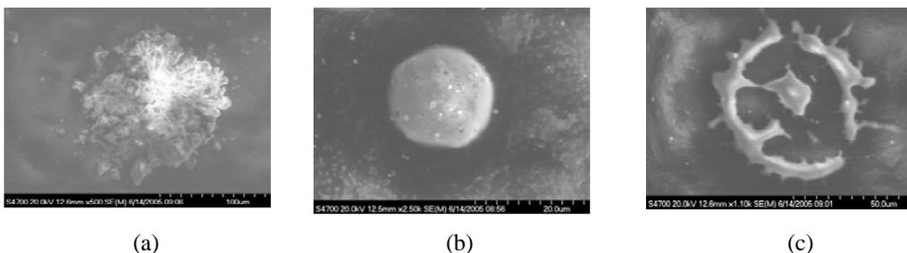
Figure 15. FE-SEM images ( $150\text{--}2500\times$  magnification) of three different types of particle morphology. Particle “a” apparently did not melt, while particle “c” apparently was melted when it hit and splattered. Particle “b” probably did not melt since it has so many Al particles coating it.
