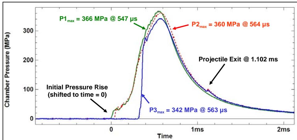
Figure 35. Pressure-time traces for small-caliber gun firing (test 065).
