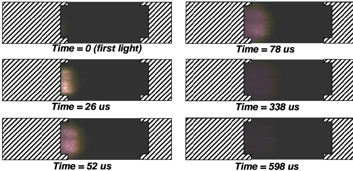
Figure 31. Flame spreading for inert propellant bed (test 046).
